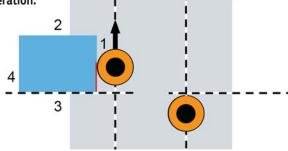
2) While the infeed operating head arrisses edge 2, the pane moves forward horizontally and the outfeed operating head begins processing edge 3.
