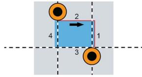
3) The outfeed operating head arrisses edge 4, moving vertically, and at the same time, the infeed operating head begins processing a new pane.
