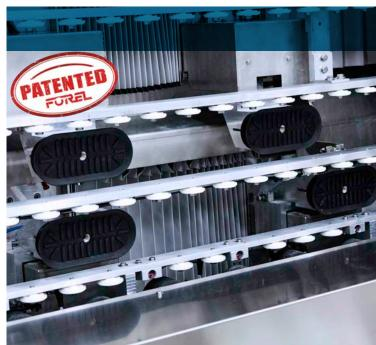
At the end of every work cycle, a **drying** system cleans and dries the suction cup to ensure a perfect hold on the next pane.
